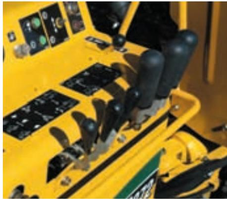
**Operator presence system.** The SC372 is equipped with three operator-sensing control levers that monitor the operator's touch and maintain cutter wheel engagement. When the operator's hands leave the control levers, an automatic disengage and braking sequence will stop the cutter wheel in less than nine seconds. With this safety system, the cutter wheel will automatically stop when the operator releases the hydraulic cutter wheel controls.
