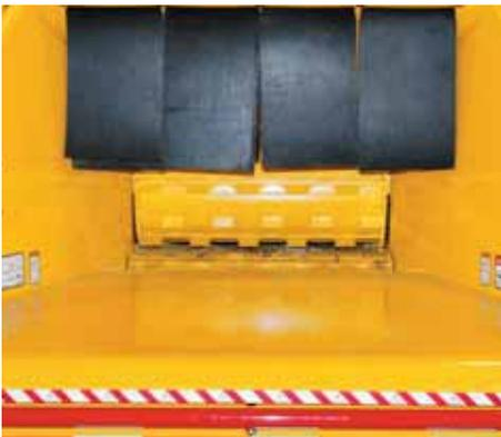
*The SmartFeed system increases operator productivity and reduces strain on vital engine parts. A patented feed sensing control system monitors engine rpm and automatically stops or reverses the rollers when feeding larger, hardwood material. Plus, it senses feed roller jams and responds by automatically shifting material back and forth, reducing the need for manually manipulating the control bar.*
