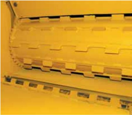
*The lower feed roller is offset from the upper feed roller by 11" (28 cm). Material is easily pulled to the upper feed roller, so there is less need to manually raise the upper feed roller for larger diameter material.*
