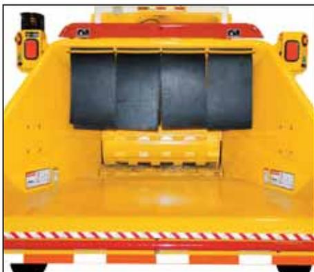
*The infeed table design is the largest in its class! It funnels material to the drum opening, allowing for smooth material feeding from table to drum. The overall table width is 72" (183 cm) with a 39" x 62" (99 cm x 157 cm) opening by the infeed curtains and a drum opening of 22" x 28" (56 cm x 71 cm).*
