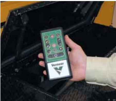
*Optional remote control lets one person do the work of two. Operate one machine to load while still maintaining control of the chipper. The remote control operates forward, reverse and stop functions of the feed rollers, restarting the feed rollers, engine throttle, engine stop, crush boost for the upper feed roller and hydraulic discharge chute positions (if equipped).*
