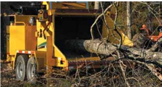
*SmartCrush puts the pressure on branches. Once the upper feed roller raises for four seconds, it will automatically increase down pressure on the material being fed. This allows the upper feed roller to easily climb onto large forked material before the increased down pressure is applied for maximum pulling force.*
